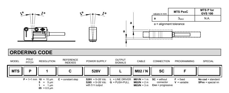
Example > MAGNETIC SENSOR MTS P 1 C 528V L M02 / N SC F
