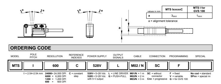
Example TMAGNETIC SENSOR MTS I 600 C 528V L M02 / N SC F
